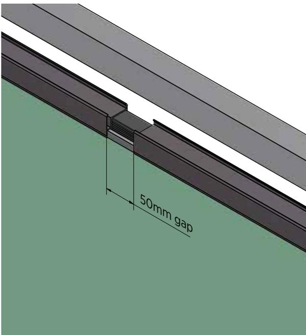
A gap of 50mm is needed to avoid LED and Handrail damage due to elongation and contraction from heat related matters.
